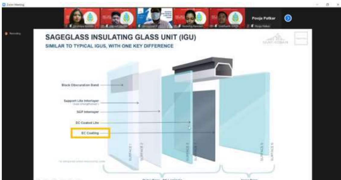
Technical session by Mr. Venugopal.R on "Energy Efficient Glasses" explaining sage glass insulating glass unit (IGU)
