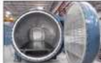
Prepreg Layup Autoclave Curing
