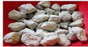
Manufactured and Engineered Truly fly-ash Aggregate with Light in weight (METAL) (Patent App. No: 202221065222 )
