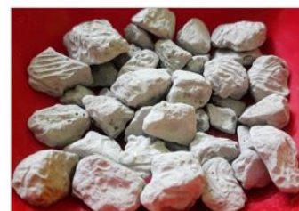
Manufactured and Engineered Truly fly-ash Aggregate with Light in weight (METAL) (Patent App. No: 202221065222 )
